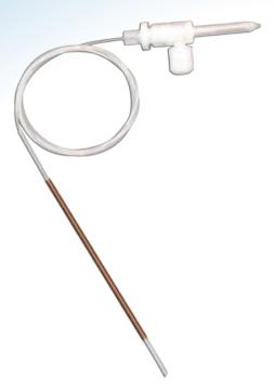
The C-Flow is a molded, fixed-capillary style PFA (perfluroalkoxy) concentric nebulizer for the introduction of low-volume (< 2 mL) samples to the Teledyne CETAC Aridus II Desolvating Nebulizer System. The inert PFA construction allows the introduction of all acids (including hydrofluoric acid), alkalis and organic solvents.
